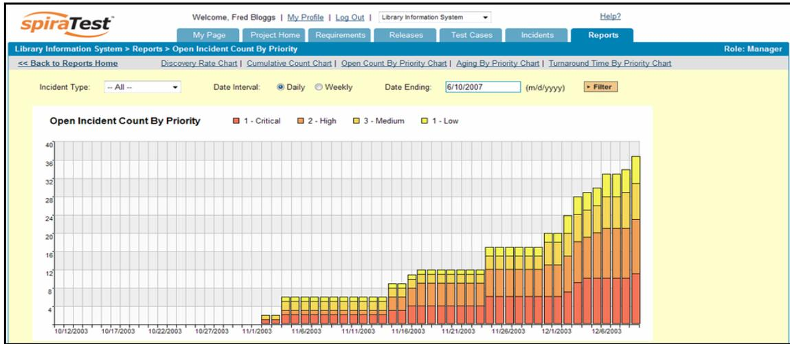
In this version of the report, the y-axis represents the number of incidents, and the x-axis represents a specific day in the time-span. The exact count of each bar in the stacked histogram can be viewed by positioning the mouse pointer over the bar, and a "tooltip" will pop-up listing the actual data value. You can also filter the type of incident being reported, as well as change the end date for the date interval.
